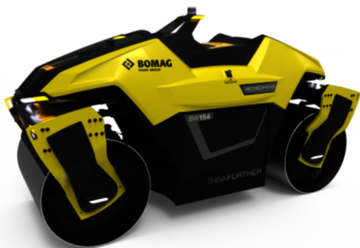
Figure 2. BOMAG Robomag Autonomous Roller
